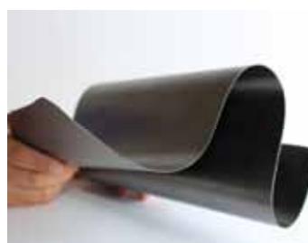
Left: high flexibility of the bipolar plate, right: stack with 4000 cm 2 cells
