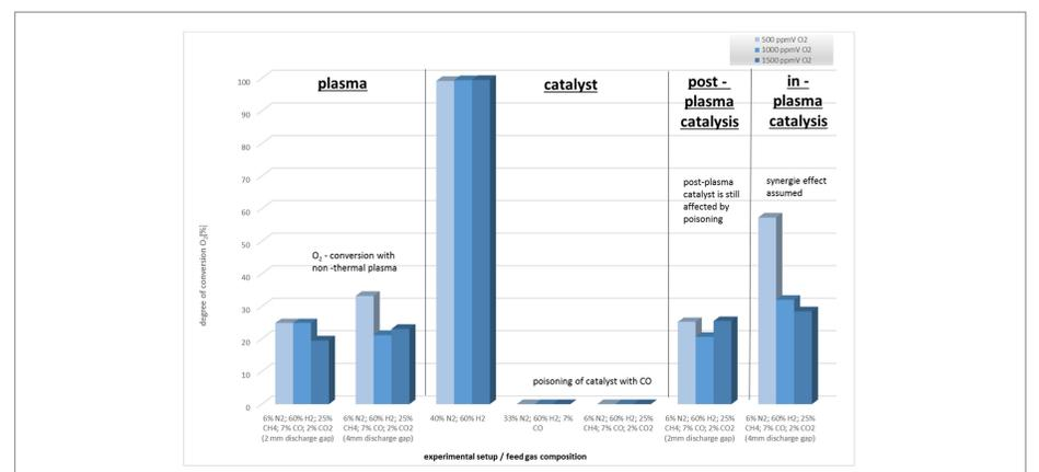
Figure 2: results of O<sub>2</sub> conversion in model steel mill gas
