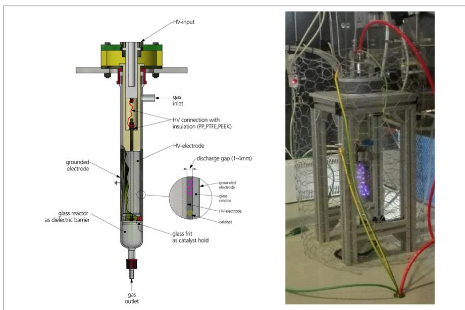
Figure 1: packed-bed DBD reactor
